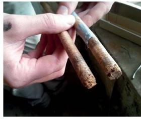
Two of the timber cores taken from a joist allowed us to date the low end to the 1420/21 felling season.
