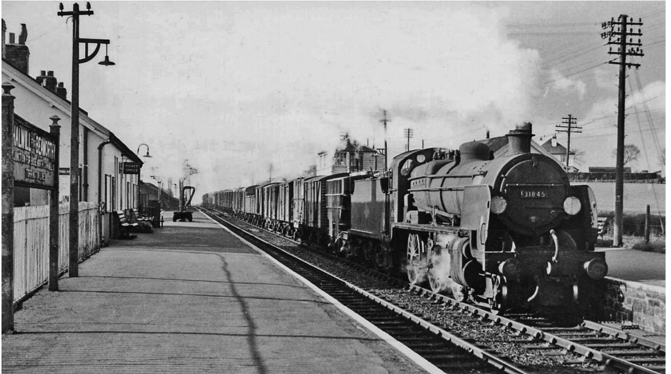
Halwill Junction station, with Up freight. View northward, towards Wadebridge and Padstow on the ex-LSW North Cornwall line, also the branches to Bude and to Torrington. The train is headed for Okehampton and Exeter, hauled by SR Maunsell N class 2-6-0 No. 31845 (built 9/24, withdrawn 9/64).
