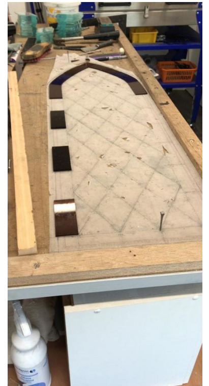
John Corley working on the glass for the windows in his Deal studio: scoring and snapping the lozenges for the cames, and painting the coats of arms for the front door.
