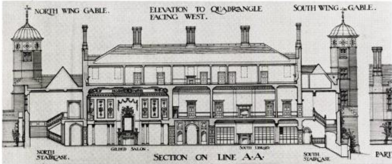
1—A SECTIONAL DRAWING OF THE CENTRE BLOCK. It shows the present State dressing room over the Wyatt vestibule in the middle, with the State bedroom over the south library
