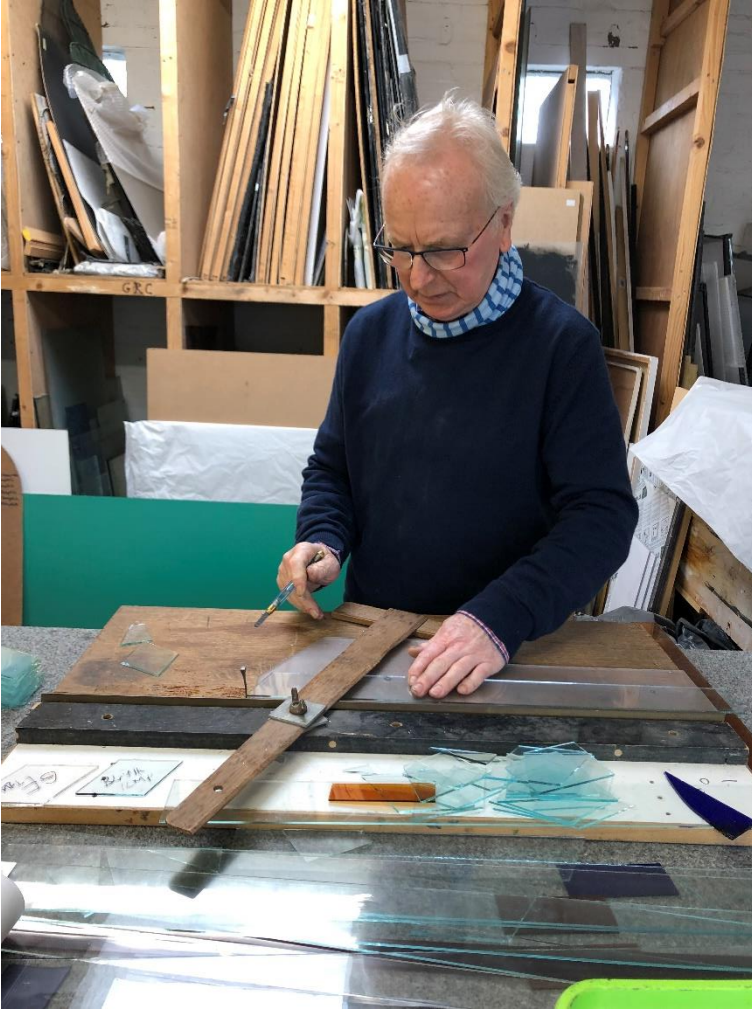
John Corley working on the glass for the windows in his Deal studio: scoring and snapping the lozenges for the cames, and painting the coats of arms for the front door.
